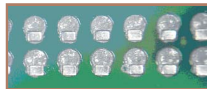
FIGURE 7: Placing rectangular segments near the through hole.
