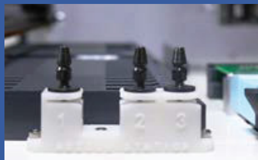
NOZZLE EXCHANGE STATION FOR MULTI NOZZLES USAGE
