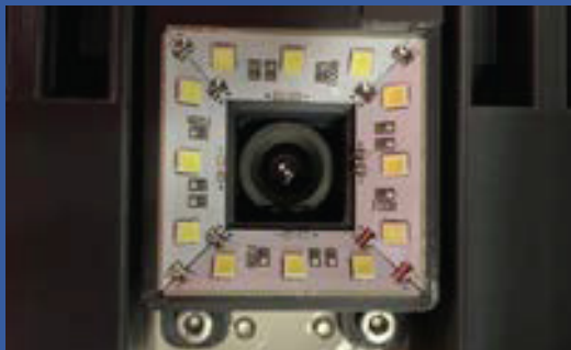
FULL VISION SYSTEM FOR FIDUCIAL AND PCB POSITION RECOGNITION
